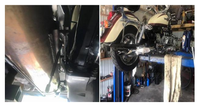
(left) Pull your spacer/shim/wrench out from between the exhaust and the mounting bracket and install the acorn nuts and tighten em down snug
