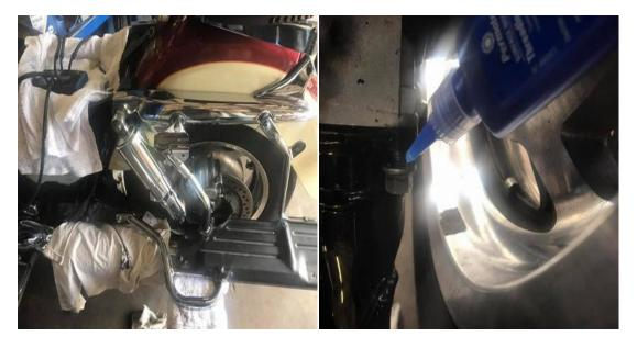
(left) Once I raise it to where the top hole lines up with the hole in the shock I bolt both tops of the shocks on and tighten the bolts. Then I raise the bike back up until the wheel is off the ground and spin the wheel making sure everything is aligned and no funny noises
