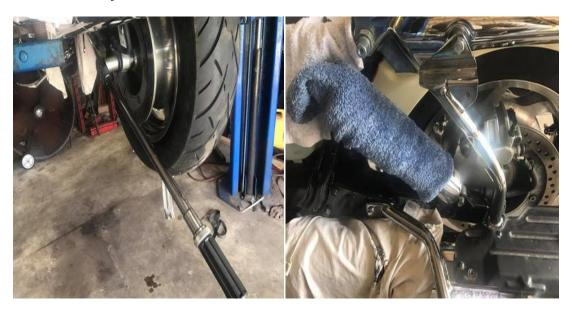
(left) At the end of Part 3 we torque the axle nut to 81 ft. Lbs.
