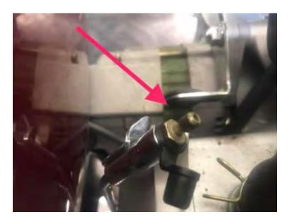
Remove the rubber cap exposing the bleeder nipple
