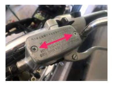
Remove the cover off the clutch master cylinder on the left side of the handlebars
