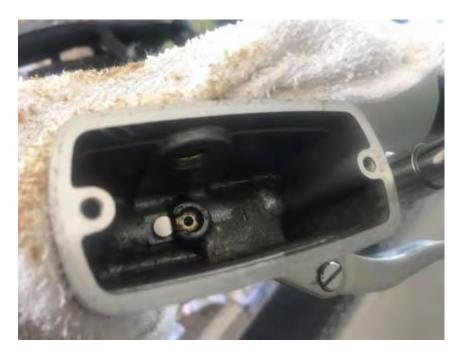
Clean the reservoir out real good and make sure the little diverter tab is in the hole in the bottom
