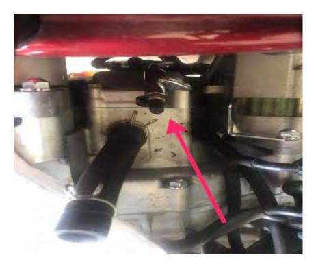
Locate the clutch bleeder nipple
