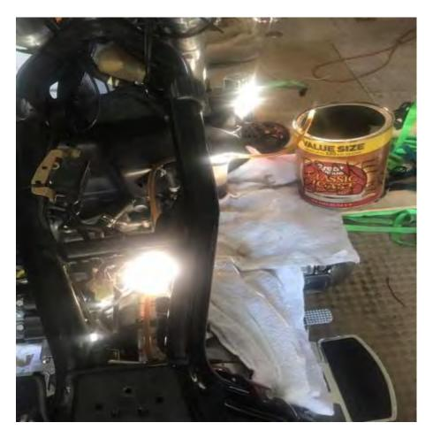
Run the tubing from the bleeder to your canister and cover all areas to keep the fluid from ruining anything it spills on
