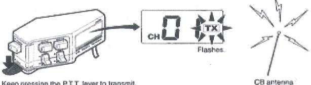
Keep pressing the P.T.T. lever to transmit.
